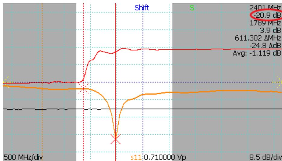
**Figure 5.4.** *S<sub>11</sub>* return loss plot (orange) and TDR trace (red) of a 2.4 GHz WiFi antenna. The return loss is calculated on the portion of the TDR trace between the cursors.
