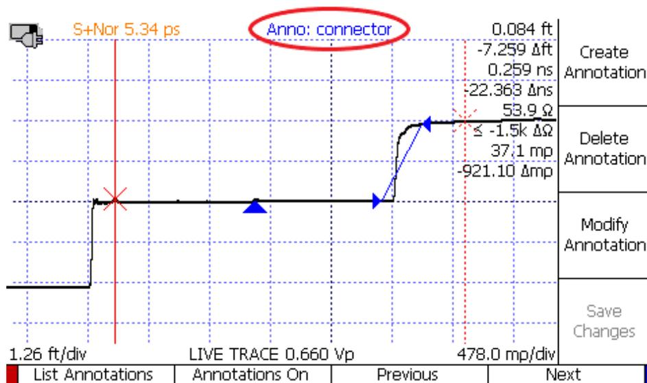
**Figure 4.29.** After an annotation is created, the multifunction indicator at the top of the screen displays the name of the currently selected annotation.
